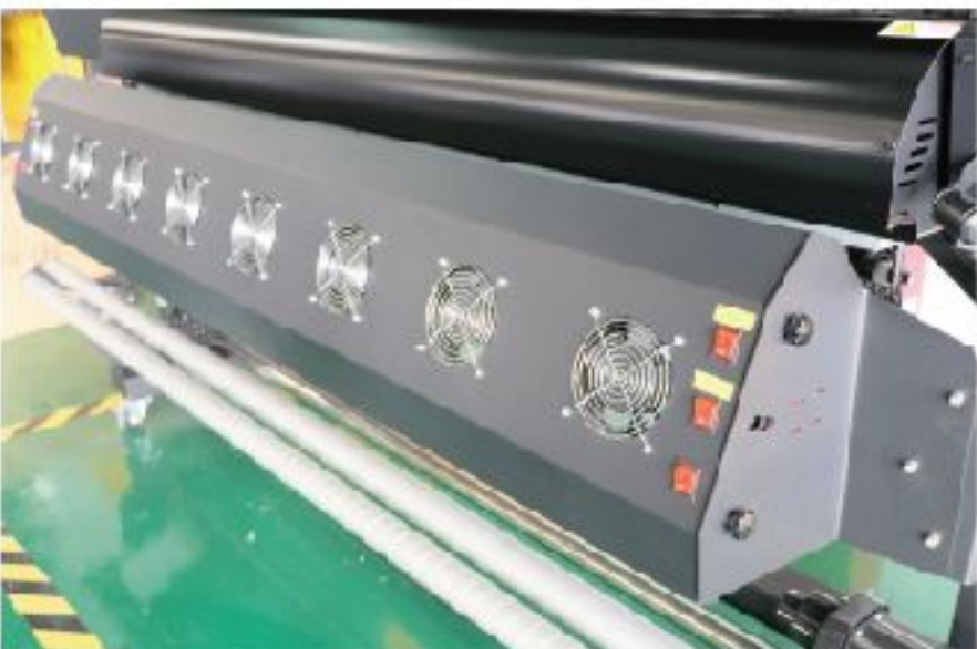
Three stage heating system including pre-heater, print heater, and rear heater and platform vacuum system with adjustable power.
