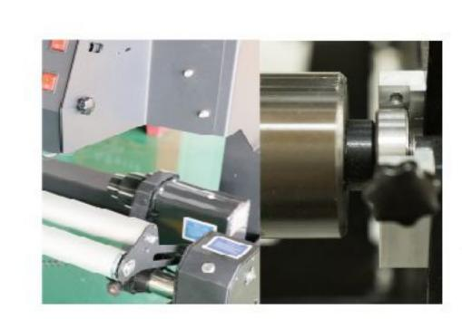
1.8m with tension take up system, intelligent rolling system. 3.2m with Inflatable take up and feed media shaft.
